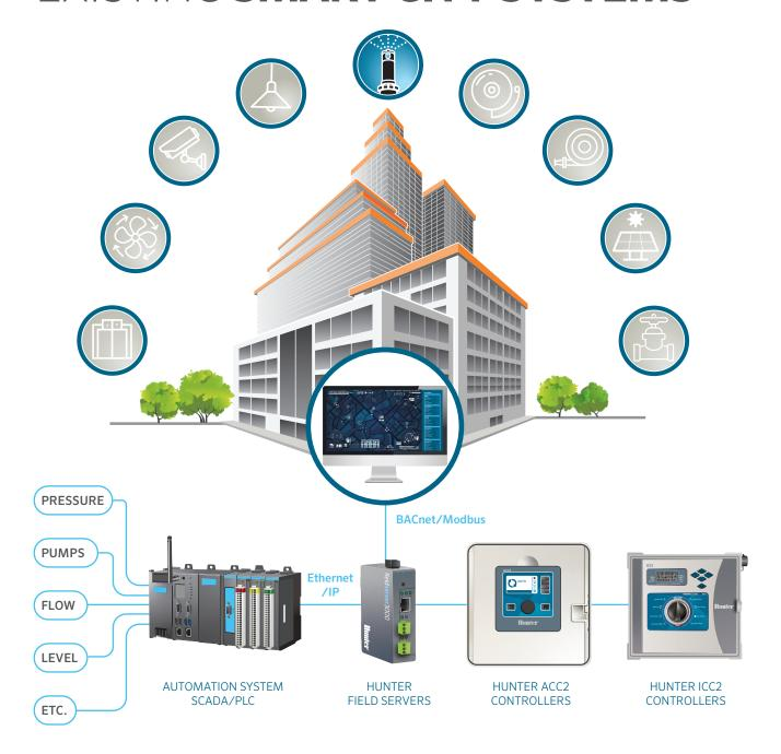
**Hunter commercial ACC2 and ICC2 Controllers** provide scalable, state-of-the-art irrigation control, leak detection, and water management when synchronised with your building management system, smart city, or wide-area SCADA applications. Multiprotocol gateways and drivers seamlessly integrate into BACnet®, Modbus®, and more than 120 other automation protocols.
