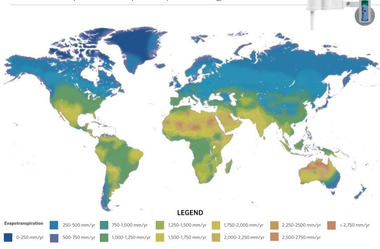
The table below will assist you in identifying the evapotranspiration (ET) region where your Solar Sync sensor is installed. There are four basic global ET regions. Each region has colour tones that correspond with average ET data for the driest season with the highest temperatures. Hunter Industries recommends choosing your region based upon average peak summer ET.
