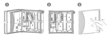
EZ-DM may also be combined with ICM-800 and ICM-400 modules for "hybrid" operation. They can use "conventional" solenoid wiring and two-wire technology at the same time, up to 54 stations maximum.
