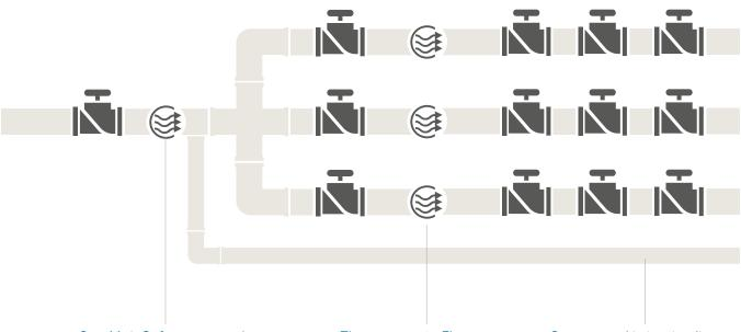
One MainSafe sensor and normally open master valve monitors the entire water source, including total monthly usage. Three separate Flow Zones schedule stations using safe, optimal target flow rates for the specific diameter of mainline pipe. One manual irrigation line provides always-on irrigation on demand, but is still monitored by the upstream MainSafe master.
