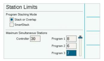
Maximum Simultaneous Stations sets a hard limit on the number of stations the controller can run at once, regardless of Flow Manager or other settings. The ACC2 Decoder Controller can run approximately 20 Hunter solenoids at once on a single output module, including P/MV outputs. The decoder controller can run up to 30 stations at once, provided they are spread over multiple decoder output modules, with not more than 20 active on each output module.
