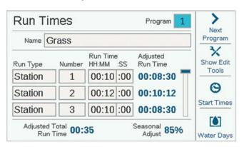
Verify that you are in the correct program, by number or name. Select the Run Type field, and select Station or Block ("Blocks" are described in detail in the Stations Menu section. Blocks replace "SSGs" in the original ACC Controller). Press the dial to select the type.
