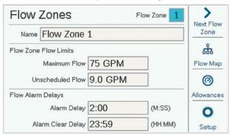
**Maximum Flow:** This sets the highest possible flow rate allowed in the Flow Zone for any reason. This should be considerably larger than the maximum flow allowed in normal irrigation (so that it does not alarm before station-level diagnostics can be performed). When the flow sensor detects a flow higher than this, the irrigation will be shut down.
