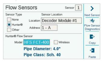
Select the sensor input number (1–6) to be set up. The controller has three Flow Sensor inputs built in, but three more can be added with the A2C-F3 Flow Expansion Module.
