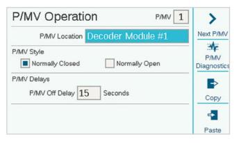
If the location is set to one of the decoder modules, the controller knows the P/MV output is assigned to a decoder on the two-wire path. If there are multiple decoder output modules, it is important to specify which Decoder Module (1, 2, or 3) it is.
