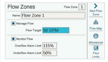
This is the only setting necessary at the Flow Zone menu for the Flow Manager function. Flow Manager will try to run enough simultaneous stations to stay at or near this rate of flow whenever there are programs available to run.
