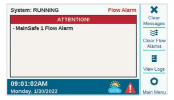
When flow alarms are detected at the Flow Zone or MainSafe level, they can be cleared from the Flow menu, Clear Flow Alarms. There also will be a shortcut soft key available to Clear Flow Alarms when these conditions are detected, after View Messages has been selected.
