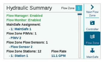
Use the soft keys to view by Controller, by Flow Zone, and by MainSafe (if applicable).
