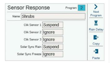
There are three standard Clik sensor inputs on the Power Supply Board. If a Hunter Solar Sync Sensor has been configured, there are also settings for Solar Sync Rain and Freeze.
