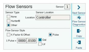
Pulse type: Enter the amount equal to a single pulse.
