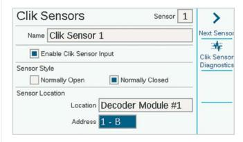
The controller sensor inputs are already configured as Normally Closed, but this can be changed for other types of contact-closure sensor inputs to Normally Open.
