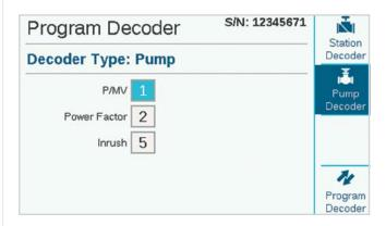
Enter the P/MV number for the decoder. This must match the P/MV assignment in the Devices menu.
