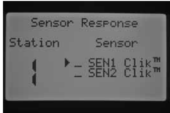
No sensor programmed for Station 1
