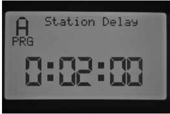
EXP: STATION DELAY FOR PROGRAM A 2 MINUTES
