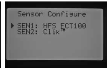
SEN 1 - FLOW SENSOR (HFS FCT100) SEN 2 - CLIK-TYPE SENSOR
