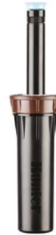
PROS-04-PRS30 Retracted height: 5⅞" Pop-up height: 4" Exposed diameter: 2¼" Inlet size: ½"
