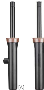
[A] PROS-06-SI-PRS30 [B] PROS-06-PRS30 Retracted height: 8¾" Pop-up height: 6" Exposed diameter: 2¼" Inlet size: ½"
