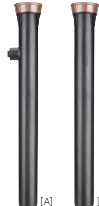
[A] PROS-12-SI-PRS30 [B] PROS-12-PRS30 Retracted height: 16⅞" Pop-up height: 12" Exposed diameter: 2¼" Inlet size: ½"
